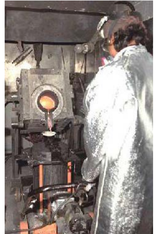
Manufacturing fuel and targets by alloying, casting and extruding
